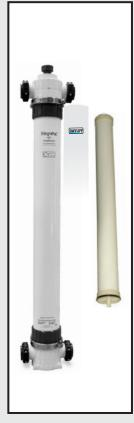
Dayliff MUF Ultra Filtration membranes are the filtering medium in ultrafiltration treatment plants for the removal of small size suspended solids and colloidal pores in raw waters including macromolecular pollutants, bacteria, viruses and microorganisms. The membranes are designed to be installed in standard pressure vessels that provide ease of operation and maintenance.
