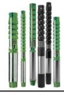
A wide range of radial and mixed-flow electric borehole pumps available in different executions and material combinations. Pumps are sized from 8'' to 16'' with motor ratings up to 400 kW that provide Flows up to  $1200 \text{m}^3/\text{hr}$  and Heads up to 600 m.
