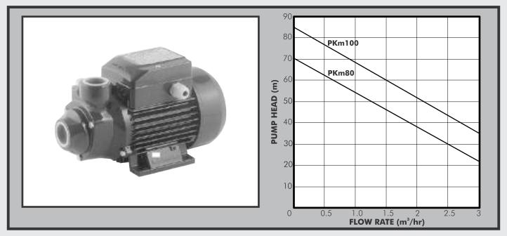
The PEDROLLO PK range of peripheral impeller booster pumps are robust, reliable and economical and used principally for water boosting in domestic and small scale water transfer applications where there is insufficient mains pressure available. The pump body is made from cast iron with a brass insert set into the front housing for improved starting performance and protection from jamming.
