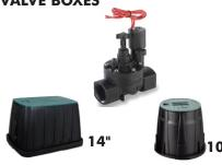
Dayliff irrigation solenoid valves are durable plastic diaphragm valves used for irrigation systems control and automation. They are available in 1",  $1\frac{1}{2}$ " and 2" sizes and F/F BSP threaded with a 24VAC solenoid. They are made from nylon plastic with all models having a manual override in case electrical automation is not required. Operating pressure range is 1.4 bar to 10 bar.
