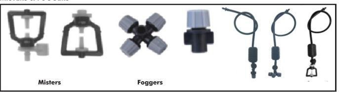
Dayliff Misters and Foggers are the ideal solution for specialised irrigation applications such as seed germination, cutting propagation, sanitization and humidity temperature control. They emit droplet sizes between 70 and 150 Micron and are suitable for both inverted an upright installations.
