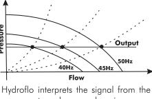
Hydrotlo interprets the signal from the pressure transducer and varies pump speed to maintain constant set pressure at various demand levels
