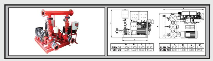
DAYLIFF FLEN packaged Fire Sets are specially designed to provide automatic water supply to fixed automatic sprinkler firefighting installations. Pump sets combine single duty diesel and electric powered supply main pumps to ensure serviceability in all conditions as well as a jockey pump to maintain system pressure. The fire sets are certified by KEBS for assembly in conformity to BS EN 12845 standard to ensure high reliability. Particular features include: -
