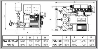
DAYLIFF FLA packaged Fire Sets are specially designed to provide automatic supply to multiple hose reel or sprinkler outlets for firefighting installations. Pump sets combine parallel duty diesel and electric powered supply pumps to ensure serviceability in all conditions as well as a jockey pump to maintain system pressure. Particular features include:-
