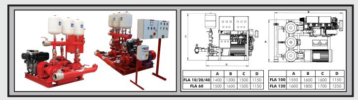
DAYLIFF FLA packaged Fire Sets are specially designed to provide automatic supply to multiple hose reel or sprinkler outlets for firefighting installations. Pump sets combine parallel duty diesel and electric powered supply pumps to ensure serviceability in all conditions as well as a jockey pump to maintain system pressure. Particular features include:-
