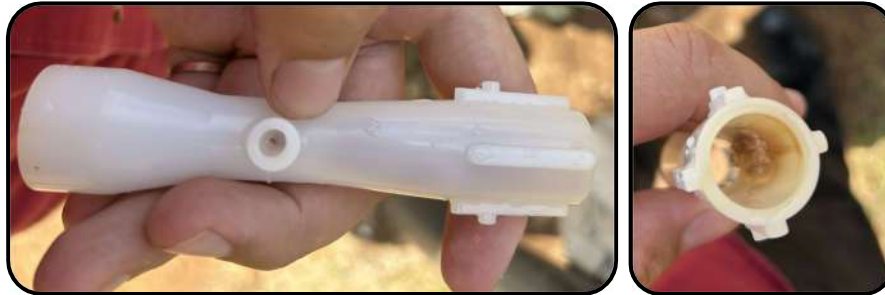
Figure 22: Example of scaling formation in Venturi
