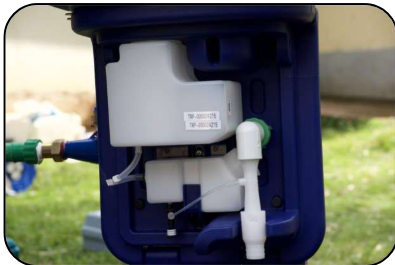
Figure 13: Chlorine refill tank, float tank, and bracket position
