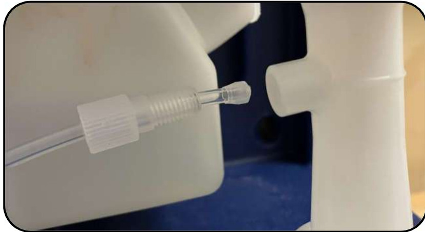
Figure 17: Compression fitting/screw and ferrule orientation on dosing tube
