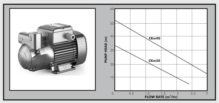
The PEDROLLO CK range are self-priming peripheral type liquid ring pumps designed for handling difficult liquids and pumping conditions. They are especially suited for irregular flow rates, aerated and foamy liquids and viscous liquids like oils and low volatility fuels and the self priming design makes them suitable for difficult suction conditions.
