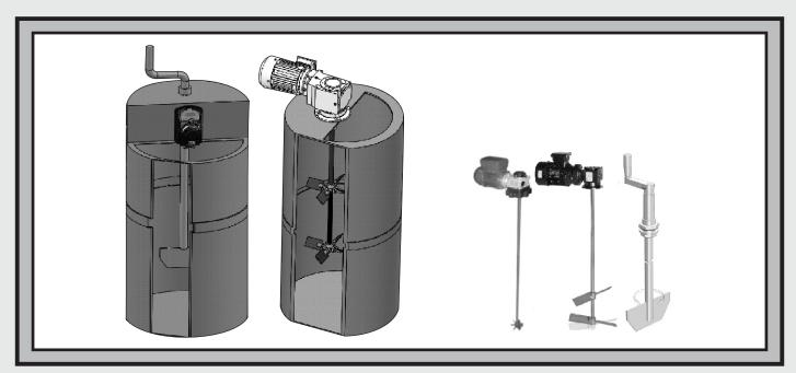
DAYLIFF chemical tanks are specially designed for use in dosing applications of various concentrate chemicals. They are made from strong corrosion resistant GRP and are available in various sizes according to applications. All are provided with a reinforced top to support a dosage pump mixer, an inspection/filling cover and a graduated chemical volume scale. A variety of dosage pumps are available to suit the dosage requirement.
