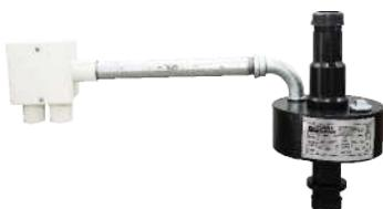
Dayliff Well heads are complete units to terminate the top of a borehole. They comprise a strong steel borehole cover plate with dipper access, drop cable/surface cable junction box and pump outlet. They are available as standard in sizes from 1 1/4" to 4" for both 6" and 8" boreholes, though other specifications are available on special order. They are supplied complete with adapter set and adapter box as loose components.
