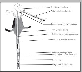
The Afridev reciprocating type hand pump has been specially designed by SKAT-HTN (Swiss Centre for Development Cooperation in Technology and Management) to meet the requirements for Village Level Operation and Maintenance (VLOM) as specified by the UNDP/World Bank. The pump has undergone extensive laboratory and field development tests and is one of only two designs which fulfils all aspects of the UNDP/World Bank specification at depths between 0 and 45m. Particular features are:
